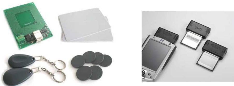
Figure 10 - RFID tags (left) and RFID readers for PDAs (right)
