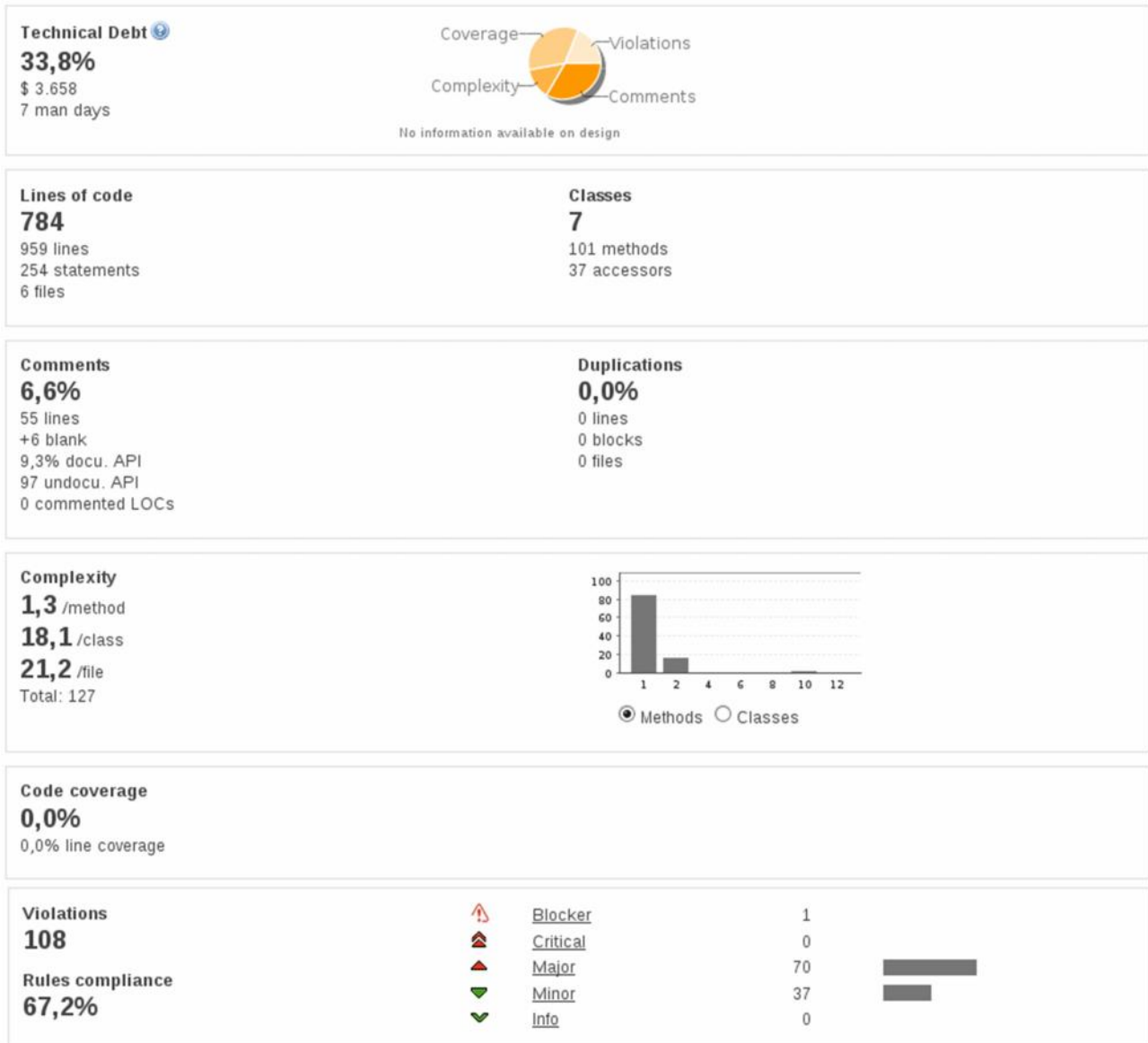
Fig. 6 Sonar results for LMStationProxy C# module
